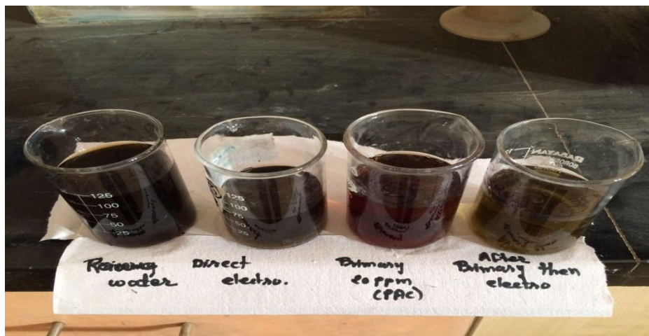
Fig. 7: Effect of lime+PAC with electrolysis (Lime-PAC dose 20, 40, 60 ppm Current: 0.8amp, electrolytes conc.:1.2 g/l, pH: 7, electrode: graphite)
